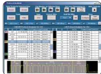
► CAN and LIN Timing and Protocol Decode.
